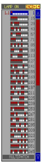
From this window, the fixture addresses are selected. The dipswitches represent address switch positions on the fixtures. New fixtures today use displays.
