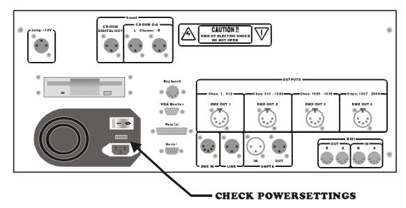
Connect the power cable to AC power
