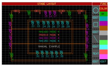
It is important that the **Pan/Tilt directions of the fixture correspond with the directions made with the trackerball.** To apply this correspondence the fixture can be turned in 9 possible positions with the keypad keys [1...9]. The fixture is now ready to be positioned somewhere on the stage by confirming its position with the left trackerball key.
